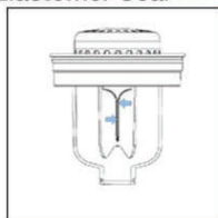
1. Elastomer Seal – Trap Shown Closed
